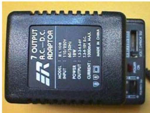
Adjustable AC to DC adaptor. The slide switch in the upper right lets you select voltages from 1.5 to 12 volts DC
